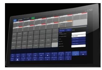
Video). It is able to interface with 3rd party systems to record and replay industry standard VGA/DVI/HDMI screen captures. The system can also record information coming from legacy interfaces such as synchronous and asynchronous serial data.
